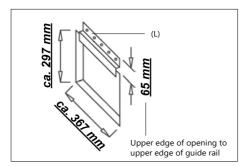
2 Check that the guide rail (L) has already been factory mounted on the cooling cabinet and, if need be, screw it on as shown in the following sketch.
