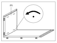
5 Position the side wall (D), ensuring that the adjusting bolts are inserted in the corresponding holes.
